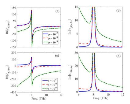
**Figure 1.** The spectral variation of the [(a), (c)] real and [(b), (d)] imaginary parts of the dielectric functions of the p- and *n*-GaAs for  $N_{p,n} = 10^{17} (\text{cm}^{-3})$  [solid curve],  $N_{p,n} = 10^{18} (\text{cm}^{-3})$  [dashed curve], and  $N_{p,n} = 10^{19} (\text{cm}^{-3})$  [dashed-157 dotted curve], respectively.
