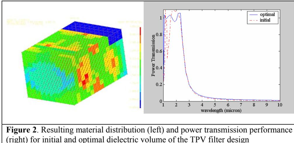
**Figure 2.** Resulting material distribution (left) and power transmission performance (right) for initial and optimal dielectric volume of the TPV filter design
