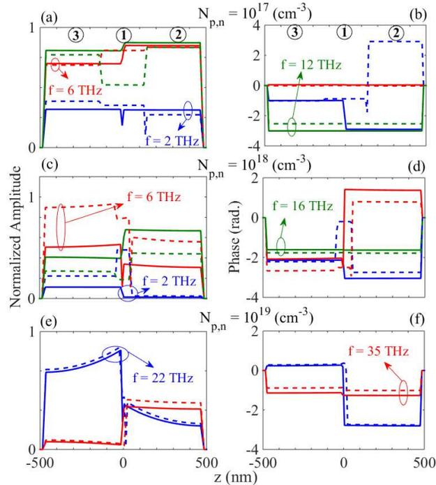
323 **Figure 4.** The normalized electric field amplitude and phase variation inside the  $pn$ -junction waveguide for
