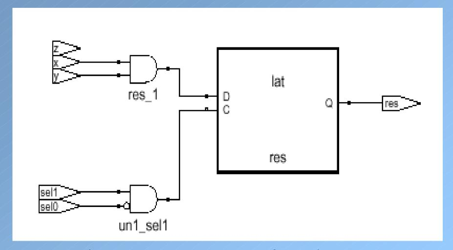
Remove the inner if-then-else from the outer one in order to infer combinational logic
