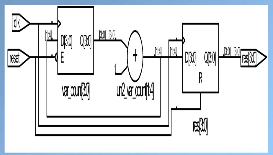
Asynchronous clear and set signal can be synthesized only if they exist in the target library.
