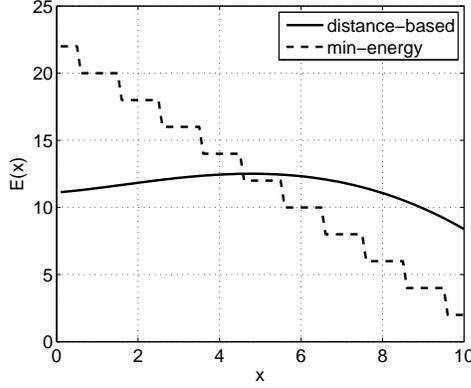
Fig. 2. Energy consumption of nodes,  $E(x)$  with distance-based routing and minimum energy routing when  $a = 0.2359, \alpha = 2, P_c = P_t = 1$ .
