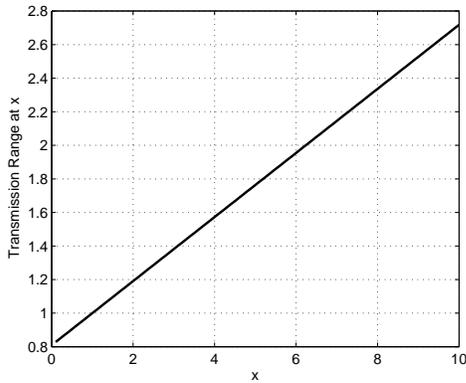
Fig. 6. Transmission ranges of the nodes with distance-based routing when  $a = 0.2359$ ,  $\alpha = 2$ ,  $P_c = P_t = 1$ .
