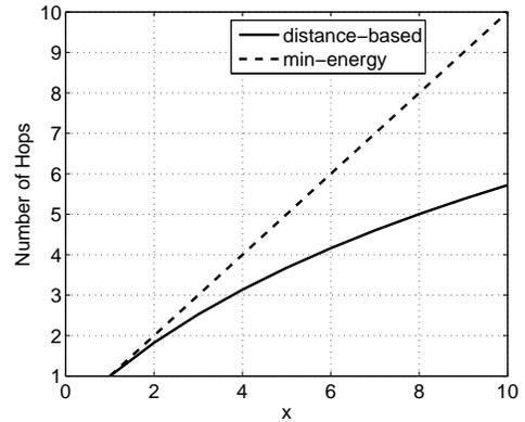
Fig. 8. Number of hops vs. distance of the node from the BS when  $L = 10$ ,  $\alpha = 2$ ,  $P_t = P_c = 1$ .
