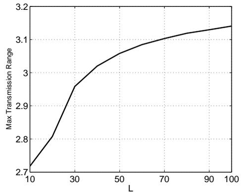
Fig. 4. Maximum transmission ranges of the nodes for varying network sizes  $L$  when  $\alpha = 2, P_c = P_t = 1$ .
